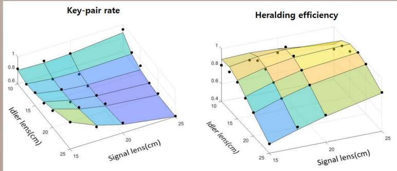
A, B and  $\gamma$  depend on the focal lengths of the pump, signal and idler lenses! [2].
