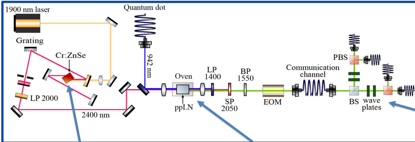
Polarisation states are encoded before being sent over various fibre links and received by Bob. Currently we statically encode states using waveplates, future work will encode on a shot-by-shot basis using an electro-optic modulator.
