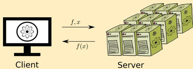
The future availability of quantum computing through remotely accessible servers pose peculiar challenges: Clients with quantum-limited capabilities want their data and algorithms to remain hidden (*blindness*), while being able to verify that their computations are performed correctly (*verifiability*).
