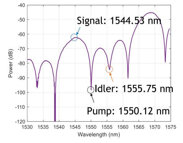
Asymmetric MZIs can filter the pump light and demultiplex the signal and idler photons.
